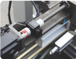
丝杆精密传动 Precision screw drive
