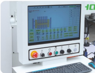
扫码后，自动显示钻头的分布 After scanning the barcode, the display will show the drill bit distribution
