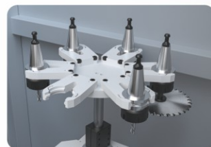
伺服圆盘六刀库 Servo rotary 6 tools magazine
