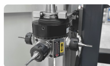
独立十字侧铣刀(选配) (K) Independent side aggregate (optional)(K)
