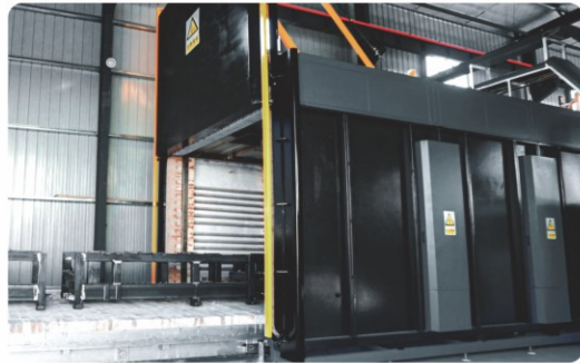
铸件去应力退火 Stress relief annealing for castings
