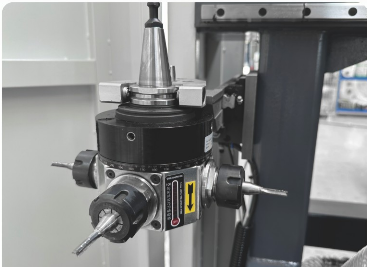
独立十字侧铣刀 (K) Independent side aggregate (K)
