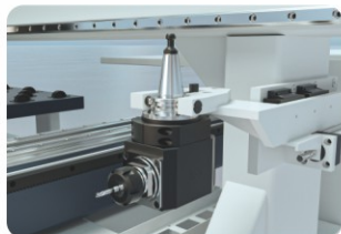
独立侧铣刀 Independent side aggregate
